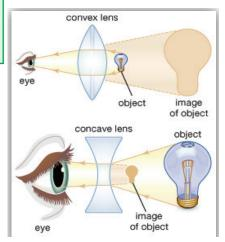
Figure 1: Convex and Concave lens
